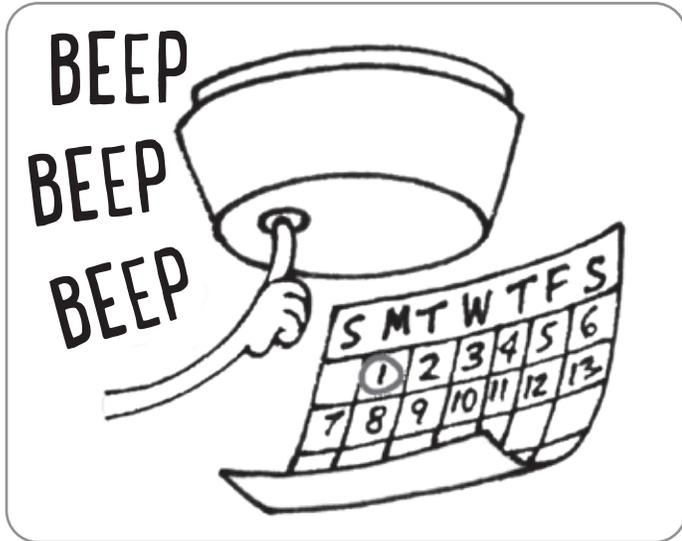
Push the test button every month. If you don't hear a sound, you need a new battery or a new smoke alarm. Fix it immediately.
