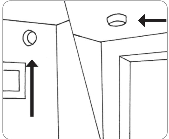
Always put smoke alarms high on the wall or on the ceiling.
