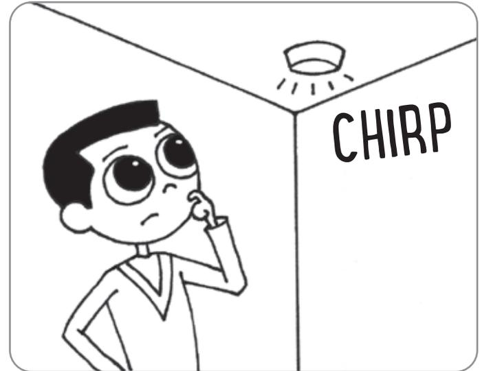
That means the battery is getting old. Replace the battery or get a new smoke alarm.
